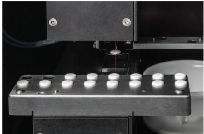
An SF measurement system uses two opposed laser beams (simulated for illustration) to scan a compacted ribbon and a tablet. In the foreground are multiple ribbon pedestals and multiple tablet "nests" that allow unattended measurement.
